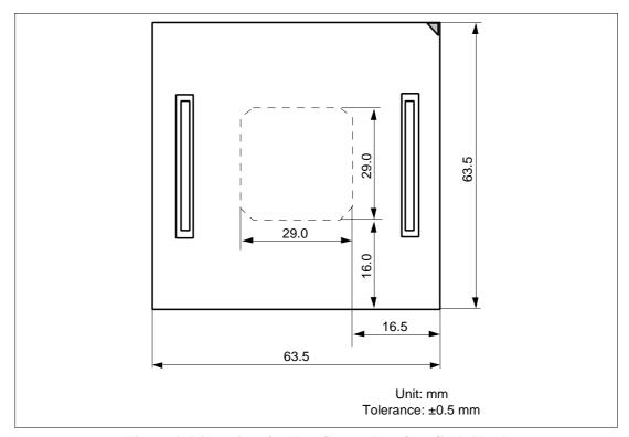
Figure 6 Dimensions for User System Interface Cable Head
